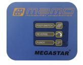
Centralized control panel allows pedal or digital punching control as well as reverse gear in the event of blockages or overloading of sheets of
